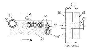
1. Floor or Wall Assembly — Min 4-1/2 in. (114 mm) thick reinforced lightweight or normal weight (100-150 pcf (1600-2400 kg/cu meter)) structural concrete. Wall may also be constructed of any UL Classified Concrete Blocks\*. Max area of opening is 300 sq in. (1935 sq cm) with max dimension of 30 in. (762 mm).
