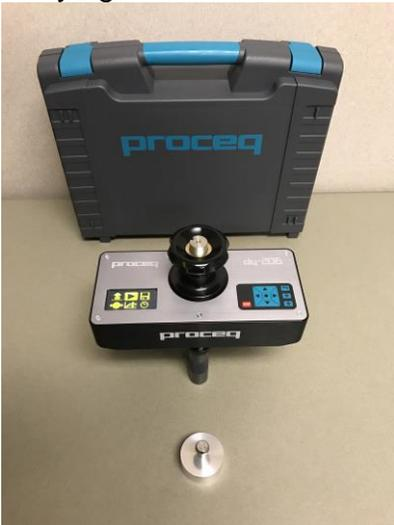
*Fig. 1 – A Proceq DY-206 Pull Tester*
