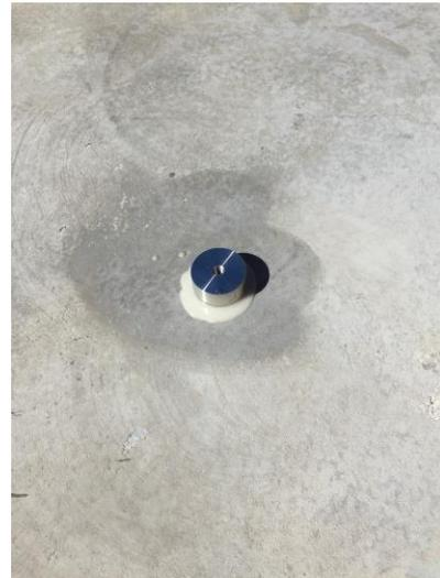
*Fig. 2 – A dolie bonded to substrate with Vulkem PUMA Primer*
