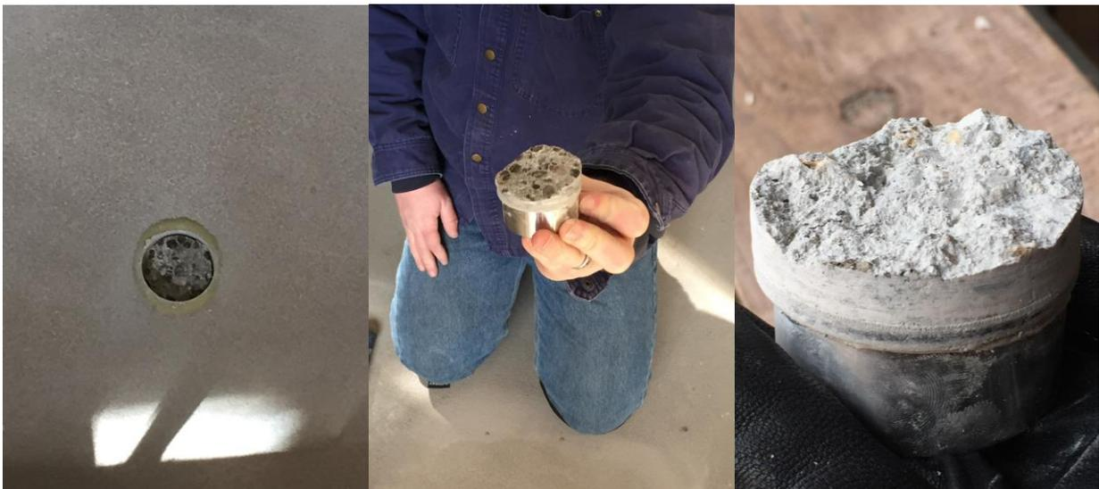
**Fig. 3 – Concrete substrate being pull tested failed prior to Tremco PUMA Primer, showing the primer's tenacious bond.**
